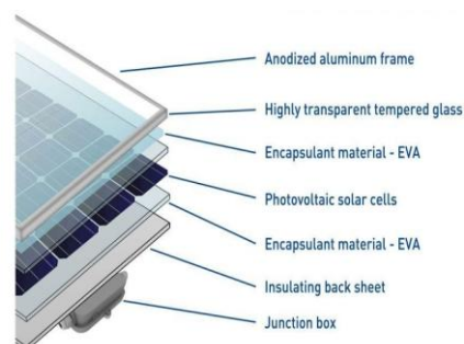
Figure 1. Structure of PV Module
