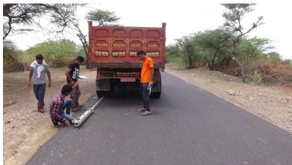
Fig. 3.4(a) Carried out BBD Test
