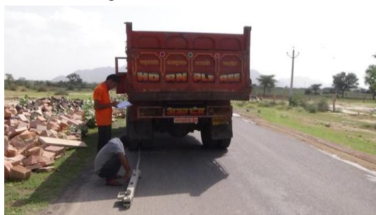
Fig. 3.4(b) Carried out BBD Test
